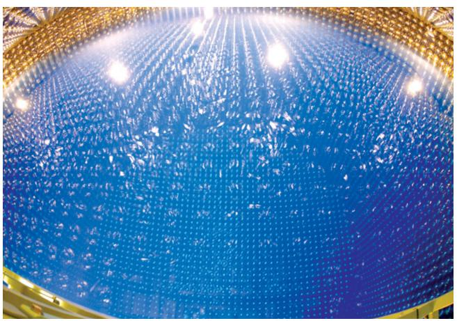
**DEEP IN A JAPANESE MINE**, the Super-Kamiokande detector uses 50,000 metric tons of water to catch neutrinos. Among the many neutrinos passing through Earth, a few collide with the water molecules, creating new particles that give off a flash of light.
